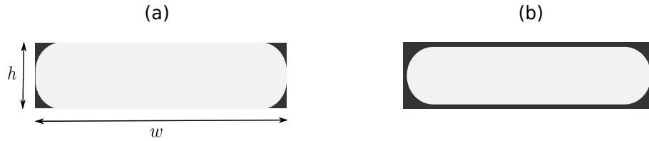
Figure 3. Sketch of the cross-section behind the liquid plug (a) when Ca \rightarrow 0 (static film deposition regime) and when (b) Ca \gtrsim Ca_c (dynamic film deposition regime). Black: liquid, white: air.
