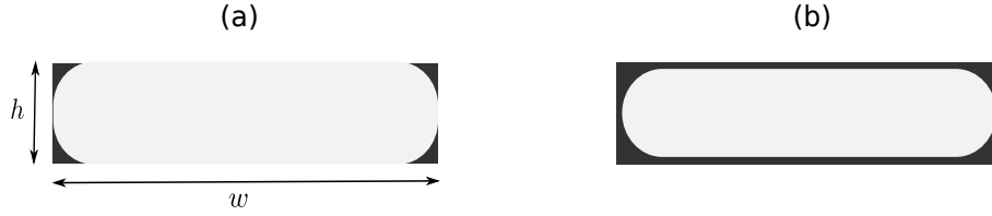
Figure 3. Sketch of the cross-section behind the liquid plug (a) when Ca \rightarrow 0 (quasi-static film deposition regime) and when (b) Ca \gtrsim Ca_c (dynamic film deposition regime). Black: liquid, white: air.
