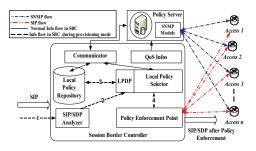
Fig. 3. Information Flow in Provisioning Mode
