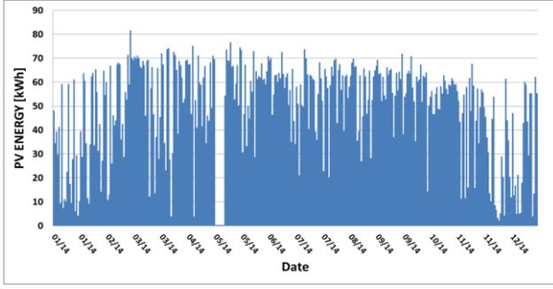
**Figure 5: Simulated PV Energy Production with P+C (ADREAM, 2014)**
