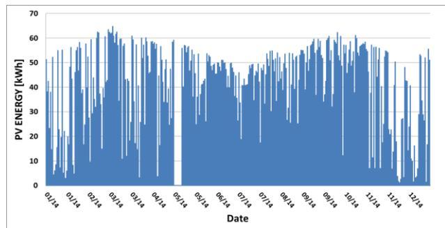
Figure 3: ADREAM's measured PV Energy Production (2014)
