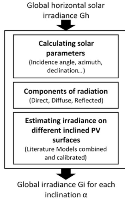
**Figure 6: Simplified diagram of the solar irradiation model**
