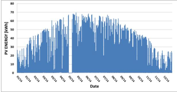
**Figure 7: Simulated PV Energy Production with Matlab (ADREAM, 2014)**
