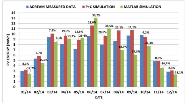
**Figure 9: Monthly Electrical Energy Production from ADREAM's PV Systems and Relative Errors for each model (2014)**
