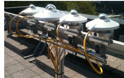
Fig. 3. Solar irradiation sensors on their inclinable stand.
