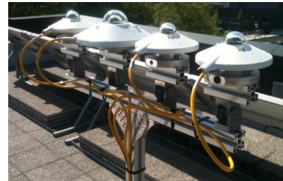
Fig. 3. Solar irradiation sensors on their inclinable stand.
