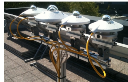
Fig. 3. Solar irradiation sensors on their inclinable stand.
