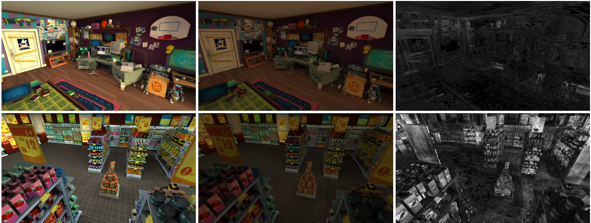
Figure 1: Examples of VPL rendering with the V-WSPD: rendered image, indirect illumination and error \times 128 . The scenes (GEEKROOM and MARKET) come from the TV Series Rabbids Invasion of Ubisoft.
