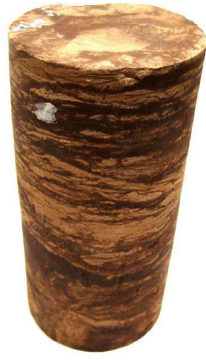
Fig. 1 Caprock sample 86 mm in diameter for a length of 180 mm.
