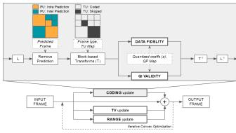
Fig. 2. A schematic view of the usage of HEVC information in the optimization framework.
