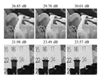
Fig. 3. Details of the up-sampled images using, from left to right, a  $Bic_8$  upsampling, the SOA approach from [10], and the proposed enhancement framework (initialized with the SOA result). PSNR values are computed on each image patch.
