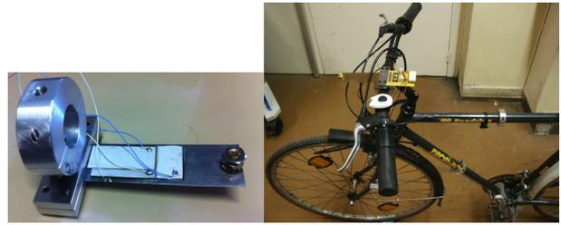
Fig. 8. Harvester with piezoelectric layer and tip mass.
