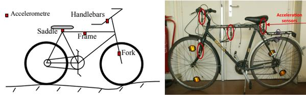
Fig. 1. Acceleration sensors mounted on a bicycle.
