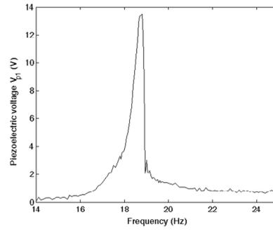
Fig. 17. Experimental frequency response result: acceleration  $2 \text{ m/s}^2$ .
