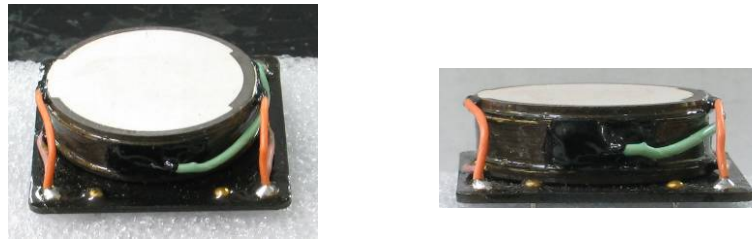
Fig. 1: Pictures of the stacked disk-type piezoelectric transformer operating in thickness mode
