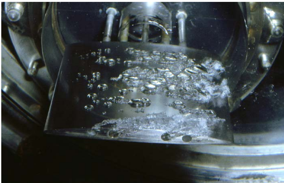
Figure 1: Typical example of cavitation on a hydrofoil. The hydrofoil is mounted in the hydrodynamic tunnel of LEGI at a positive angle of attack. Flow of water is from left to right. Chord length is 10 cm. Cavitation bubbles originate from microbubbles or cavitation nuclei carried by the liquid flow. They are activated by the low pressure region that exists near the leading edge of the hydrofoil. They grow to macroscopic cavitation bubbles before collapsing more downstream in the region where the pressure is recovered.
