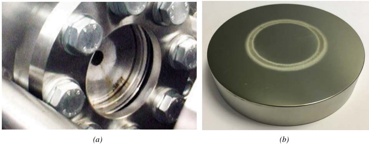
Figure 9: Example of a cavitation erosion tunnel using a radially diverging axisymmetric test section. (a) Visualization of the attached cavity. Nozzle diameter is 16 mm. (b) Typical example of an eroded specimen. Erosion is concentrated on a ring that corresponds to the closure region of the cavity shown in (a). Specimen diameter: 100 mm (LEGI Prevero facility).
