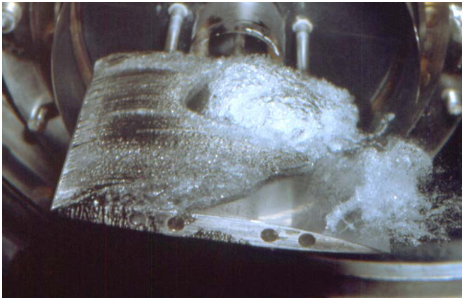
Figure 3: Typical example of attached cavitation. The cavity detaches from the leading edge of the hydrofoil. The cavity closure region is very unsteady and sheds, more or less periodically, clouds of vapor bubbles that are known to be particularly aggressive from an erosion viewpoint (LEGI hydrodynamic tunnel).
