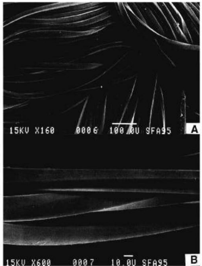
Figure 2. Scanning electron photomicrographs of the back of the supercritical fluid extraction cleaned fabric showing the absence of visible contaminants adhering to the surface of the filaments (original magnifications, A: \times 160 , B: \times 600 ).
