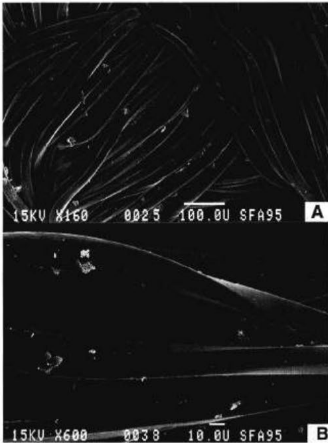
Figure 1. Scanning electron photomicrographs of the face of the control knitted fabric showing the presence of contaminants adhering to the surface of the polyester filaments (original magnifications, A: \times 160 , B: \times 600 ).
