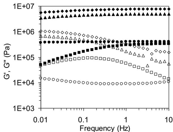
**Figure 6.** Rheological properties of PDMS(30)-g-BuP (◆, ◇), PDMS(13)-g-BuP (▲, △), BuP/PDMS(29)/BuP (●, ○), and PDMS(10)-g-BuP (■, □) at 30°C. Elastic modulus  $G'$  (full symbols), loss modulus  $G''$  (hollow symbols).
