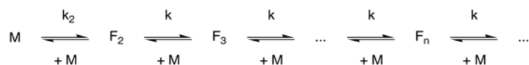
Figure 6. Association equilibria between monomer (M) and filaments (F n ) of degree of polymerisation (n).
