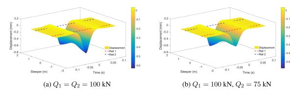
Figure 3: Displacement of sleeper for the same loads and different loads on two rails
