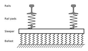
Figure 2: Dynamic model of a sleeper
