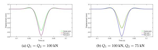
Figure 4: Sleeper displacement under the moving charge at 3 positions : middle point (green curve), the first rail seat (red curve) and second rail seat (blue curve)
