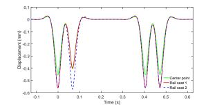
(b) At 3 positions : middle point (green curve), the first rail seat (red curve) and second rail seat (blue curve)
