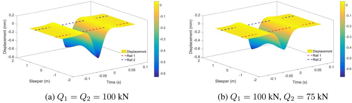
Figure 3: Displacement of sleeper for the same loads and different loads on two rails
