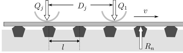
Figure 1: Periodically supported beam subjected to moving loads
