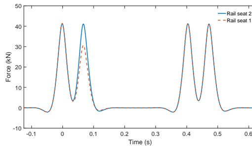
Figure 8: Reaction forces at two rail seats
