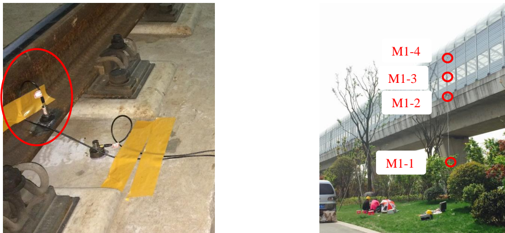
(a) The piezoelectric acceleration sensor adhered on the rail foot (b) The microphones mounted on a standing pole
