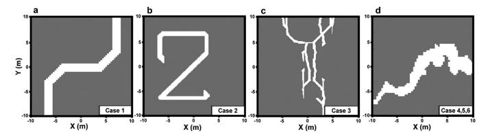
Figure 6. Presentation of the four different structures tested in the six study cases in this paper. (a) The case 1 is a linear inversion of a simple geometry to show how the optimization works. (b) The case 2 is a linear inversion of a more complex geometry. (c) The case 3 is a linear inversion of a complex multidirectional linear structure. (d) The cases 4–6 are linear, nonlinear, and joint inversion of a geostatistical generated geometry, appearing as a more natural structure.
