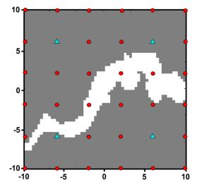
**Figure 12.** Map of the positioning of the wells for the hydraulic tomography inversion for the study case 4. The circles are the position of the measurement piezometers and the triangles are the position of the pumping wells.
