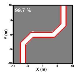
**Figure 8.** Comparison of the optimal structure found by inversion (in white) and the true structure (bold boundaries) for the case study 1. For this simple geometry, the inverse algorithm could easily reproduce the structure.
