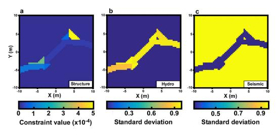
**Figure 17.** Uncertainties analysis for the joint inversion of the study case 6. The structural constraint in (a) indicates where the structure of the model is well-constrained by a low value, and at the opposite, a high value indicates an uncertainty for its subspace direction. The properties uncertainties for (b) the hydraulic transmissivity and (c) the seismic velocity are quantified by a standard deviation on the inverted values.
