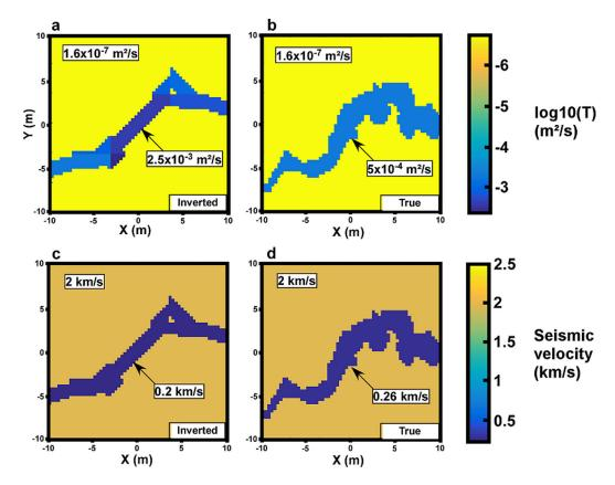
**Figure 15.** Result of the joint inverse modeling of the study case 6. The inversion finished after seven iterations. This figure shows (a) the hydraulic model, (c) the seismic model, and (b, d) the true models. The geometry of the structure in the models was optimized through a joint inversion of seismic and hydraulic data.
