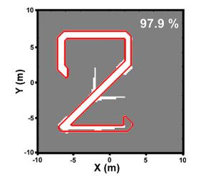
**Figure 10.** Comparison of the optimal structure found by inversion (in white) and the true structure (bold boundaries) for the case study 2. The optimization process reproduced a good structural inversion. The few inversion errors in the center of the model were lightly balanced by the inversion on the properties (see Figure 9).
