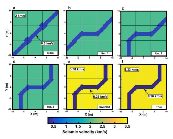
**Figure 7.** Result of the linear inverse modeling of the case study 1. The inversion finished after four iterations. This figure shows all different iterations of the inversion from (a) initial model to (e) inverted model. The true structure is shown in Figure 7f. Figure 7d corresponds to the structural optimization and Figure 7e to the properties optimization for this structure. The different CA subspaces of the model are highlighted by the black lines.
