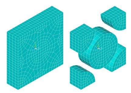
Fig. 4. FE model of the RVE, micro-scale.
