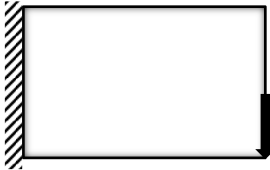
Figure 2: The proposed benchmark – In-plane dimensions: w = 320\text{mm} , h = 200\text{ mm} . Thickness: t = 2\text{ mm} . Material: E = 72000\text{ MPa} , \nu = 0.33 . Load: P = 1000\text{ N} .
