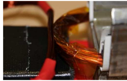
Figure 18. Detail of phase-to-phase motorette test set-up
