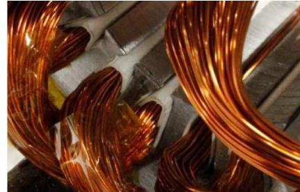
Figure 19. Detail of phase-to-ground insulation.
