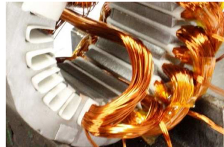
Figure 12. Details of turn distribution during coils insertion
