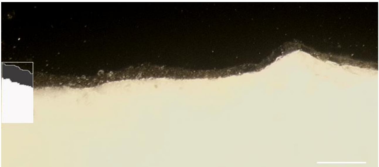
Figure 4. Polished cross section and stratigraphic scheme of sample 1 (bar 100 µm) showing the presence of just one finishing layer.
