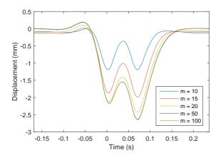
${f Fig.~7}$  Numerical results with different numbers of harmonics for the bilinear foundation
