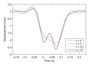
${f Fig.~6}$  Numerical results with different numbers of iterations for the bilinear foundation
