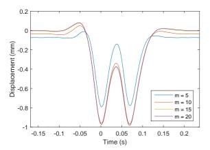
Fig. 4 Numerical results with different numbers of iterations for the cubic-nonlinear foundation
