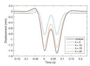
Fig. 3 Analytic solution and numerical results with different numbers of iterations for the linear foundation
