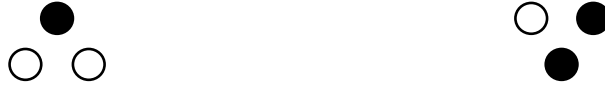
Figure 2: In this simple case, where k=3 , the set of black dots and the set of white dots have small Hausdorff distance but define two NN quantizers, say q_1 and q_2 , for which F_1(q_1, q_2) is large.
