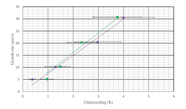
**Fig. 4.** Growth rate as a function of the undercooling. Points corresponding to pure silicon and silicon containing C and O are respectively in green circles and in purple triangles.
