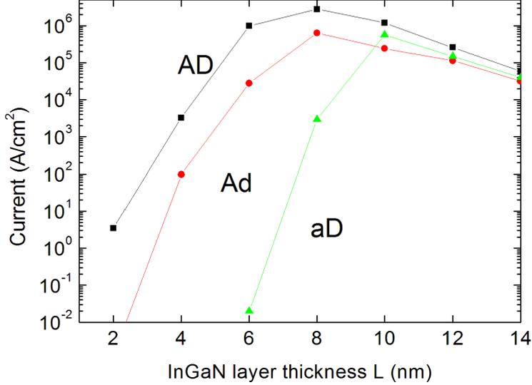
FIG. 2. Calculated current density at  $V = -1$  V in the tunnel junction GaN/In<sub>0.33</sub>Ga<sub>0.67</sub>N/GaN *versus* the thickness of the InGaN layer for the three dopings **AD** ( $N_A = 10^{19}$  cm<sup>-3</sup>,  $N_D = 10^{20}$  cm<sup>-3</sup>), **Ad** ( $N_A = 10^{19}$  cm<sup>-3</sup>,  $N_D = 10^{19}$  cm<sup>-3</sup>) and **aD** ( $N_A = 10^{18}$  cm<sup>-3</sup>,  $N_D = 10^{20}$  cm<sup>-3</sup>).
