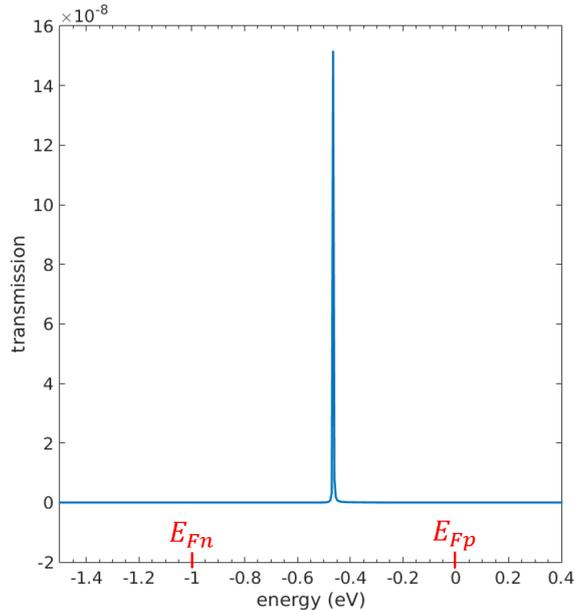
FIG. 4. Transmission with respect to the energy for the tunnel junction **Ad** with  $L = 6$  nm and  $x = 0.33$ . The peak corresponds to the energy of the lower localized state shown by the orange arrow in Fig. 3(a). Almost all the current flows through this localized state.
