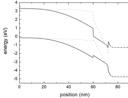
FIG. 6. Band diagrams of the cell **aD** with  $L = 12 \text{ nm}$  without polarizations (solid line) and with polarizations (dash line). The polarizations limit the SCR at the InGaN layer while without polarizations such a SCR largely over gone in the p-type GaN which has a low doping.
