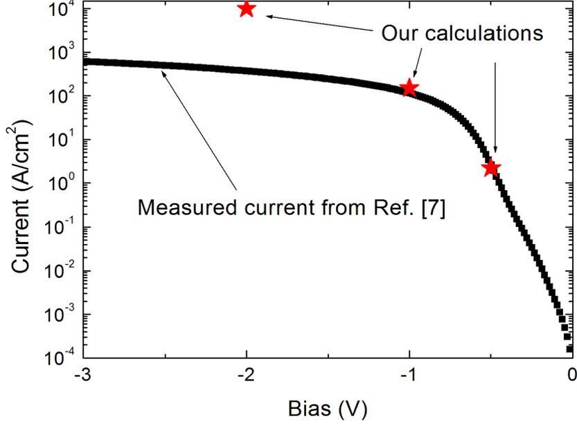
FIG. 1. Current characteristics of the diode (extracted from Ref. 7):  $N_D = 5 \cdot 10^{18} \text{ cm}^{-3}$ ,  $N_A = 10^{19} \text{ cm}^{-3}$ , the In content  $x=0.33$  and the InGaN layer thickness  $L=6.4 \text{ nm}$ . Crosses represent our calculations.
