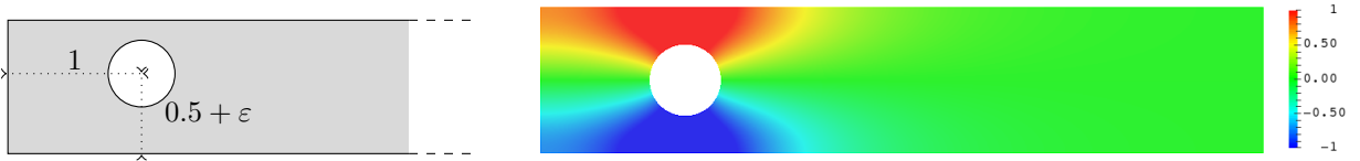
Figure 12: Left: geometry of \Omega_+^\varepsilon . Right: real part of a trapped mode for \varepsilon = 0 and k^0 := \sqrt{\lambda^0} \approx 2.7403 .
