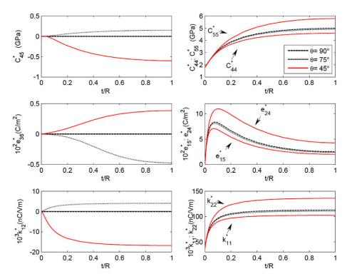
**Figure 8.** Three different cell arrangements are considered, that is,  $\theta = 90^{\circ}$ , 75°, 45° for the study of the influence of parallelepiped arrays on the effective properties behavior.
