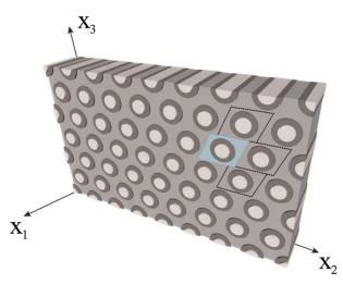
Figure 1. Three-phase periodic composite reinforced by fibers.
