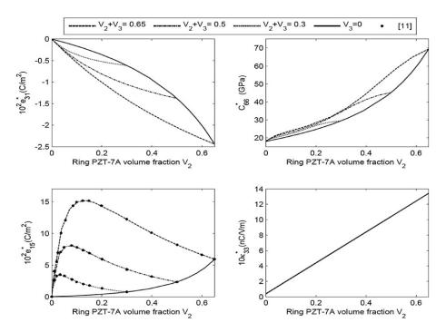
**Figure 6.** The effective piezoelectric coefficient  $e_{31}^*$ ,  $C_{66}^*$ ,  $e_{15}^*$  and  $\kappa_{33}^*$  for a composite with ring-shaped cross-section and hexagonal periodic cell are calculated by the present model. In particular,  $e_{15}^*$  coincides with the equivalent coefficient reported in Xu *et al.*, [6].
