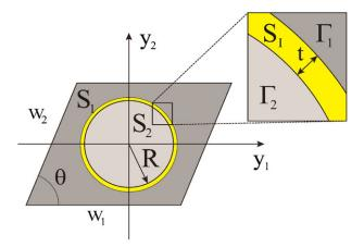
Figure 2. Composite consists of a parallelepiped array of two circular and concentric infinitely long fibers.
