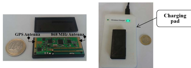
Figure 15. Tracking patch with waterproof packaging and integrated wireless charger.
