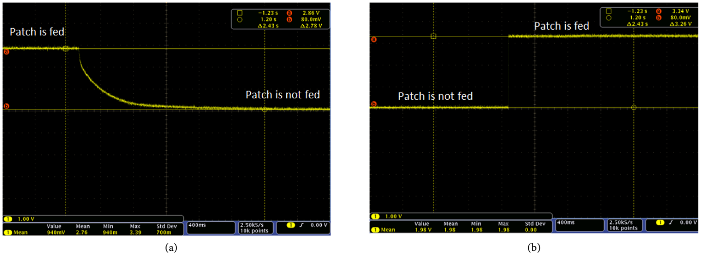
Figure 21. Undervoltage protection ((a) deactivation @ Vbat = 2.86 V and (b) activation @ Vbat = 3.34 V).
