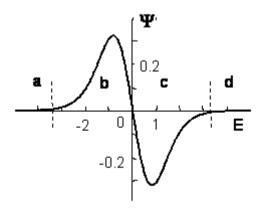
Fig. 5. Mean number of open equivalent channels  $\Psi$  as a function of normalized transmembrane energy E. As  $\Psi$  is positive (part "b"), then the open inward channel number is larger than the open outward channel number. The total ion flux is inwardly. As  $\Psi$  is negative (part "c"), the total ion flux moves outward through the membrane.
