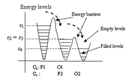
Fig. 2. Closed-open transitions. An energy  $\Delta\epsilon$  arriving in a closed channel causes energy barrier decay. F1: energy levels of an equivalent charge of a closed inward channel  $C_i$ . O1: energy levels of an equivalent charge of an open inward channel  $C_i$ . F2: energy levels of an equivalent charge of a closed outward channel  $C_o$ . F2 is the same that O1. O2: energy levels of an equivalent charge of an open outward channel  $C_o$ .
