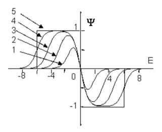
Fig. 6. Variation in wavelet with parameter value  $E_2$ . Curve 1:  $E_2 = -1.5$ ; curve 2:  $E_2 = -3$ ; curve 3:  $E_2 = -4.5$ ; curve 4:  $E_2 = -6$ ; curve 5: Haar function.
