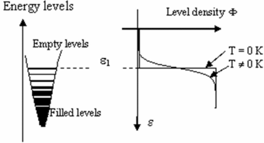
Fig. 3. Energy level distribution. At the temperature  $T = 0$  K, the energy  $\varepsilon_1$  is the border between the filled levels and the empty ones. Then the level density curve exhibits a step at  $\varepsilon_1$ . If the temperature is  $T \neq 0$  K, there are some filled levels above this energy.
