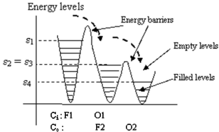
Fig. 2. Closed-open transitions. An energy  $\Delta\varepsilon$  arriving in a closed channel causes energy barrier decay. F1: energy levels of an equivalent charge of a closed inward channel  $C_i$ . O1: energy levels of an equivalent charge of an open inward channel  $C_i$ . F2: energy levels of an equivalent charge of a closed outward channel  $C_o$ . F2 is the same that O1. O2: energy levels of an equivalent charge of an open outward channel  $C_o$ .
