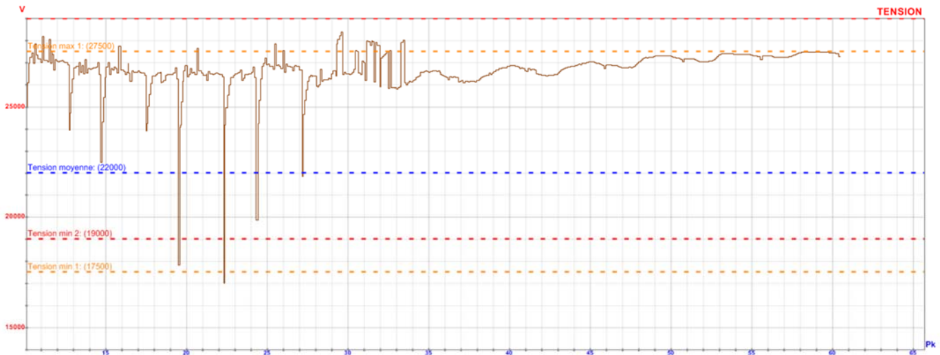
Fig. 6 : Line voltage versus train position, for one of the eight running trains
