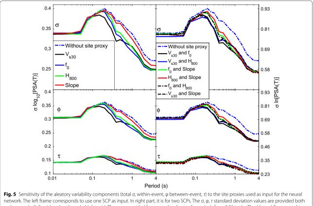
network. The left frame corresponds to use one SCP as input. In right part, it is for two SCPs. The  $\sigma$ ,  $\varphi$ ,  $\tau$  standard deviation values are provided both on log<sub>10</sub> scale (left axis) and on ln scale (right axis). They are provided for spectral ordinates for periods from 0.01 to 4 s. The  $M_w$  and  $R_{JB}$  are used to obtain the reference model (without proxies in this figure for the one SCP and two SCPs)
