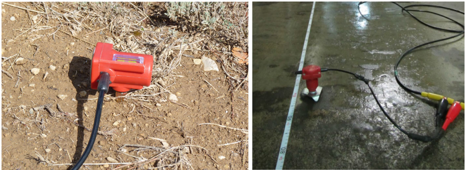
Fig. 5 Examples of 4.5 Hz geophones. Left horizontal geophone with a spike pressed in soil. Right vertical geophone mounted on tripods for a good contact on stiff surfaces
