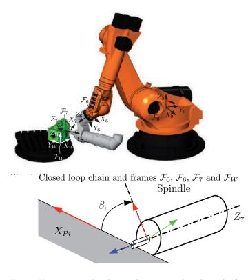
Fig. 5. Kinematic redundancy characterized with angle  $\beta_i$
