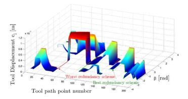
Fig. 8. Tool displacement  $c_i$  [m] as a function of the tool path point number and  $\beta$  angle for the best workpiece placement. The green curve characterizes the optimum redundancy planning scheme, i.e.,  $\beta_{opt}$  vector, whereas the red curve represents the worst redundancy planning scheme for this workpiece placement
