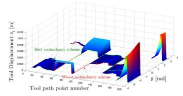
Fig. 10. Tool displacement  $c_i$  [m] as a function of the tool path point number and  $\beta$  angle for the worst workpiece placement. The green curve characterizes the optimum redundancy planning scheme, whereas the red curve represents the worst redundancy planning scheme for this workpiece placement
