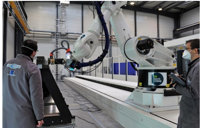
Fig. 1. KR500 L480-2 MT mounted on rail located at IRT Jules Verne
