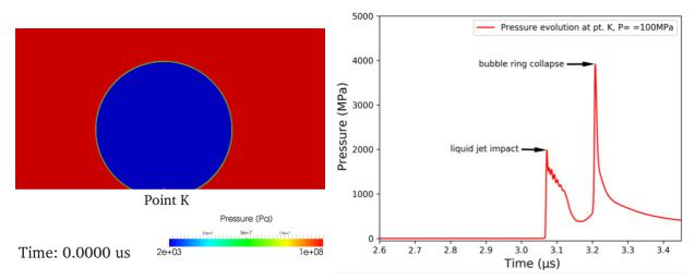
Figure 3a (left) : : Initial bubble setup with represented point K in the bottom solid boundary where pressure evolution is plotted; Figure 3b(right): Pressure evolution at point K in the bottom solid boundary,  $R_{max} = 500 \ \mu m$ ,  $\gamma = 0.8$ ,  $P_{\infty} = 100 \ MPa$
