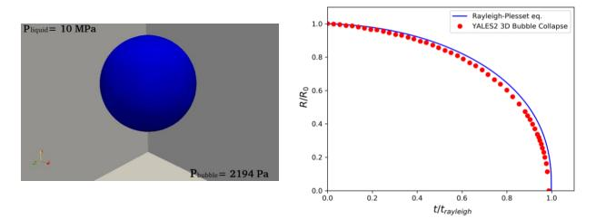
Figure 2 :Simulation of a single 3D spherical bubble collapse with YALES2 and comparison with Rayleigh Plesset collapse model for  $R_{max} = 500$  $\mu m$ ,  $P_{\infty} = 10$  MPa. Numerical bubble collapse setup (left); evolution of non-dimensional radius with respect to non-dimensional time (right)
