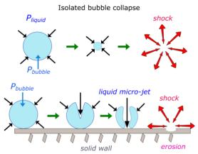
Isolated bubble collapse near a solid boundary
