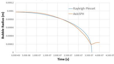
Figure 2. Comparison of bubble radius vs. time, SPH against Rayleigh-Plesset solution for a bubble collapse simulation (domain shown in figure 1)
