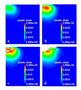
Figure 5. Sequence of images from damage simulation of a stainless steel A-2205 specimen, (a) Shows the plastic strain accumulation in material without damage, (b) high plastic strain zone just beneath the top surface, (c) damage initiation from the point of highest plastic strain, (d) material loss due to a single indent (domain size shown in the figure is same as in figure 3)
