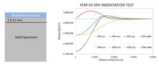
Figure 4. FEM results are compared against SPH for indentation of 6 microns in depth and 0.4 mm in radius for a stainless steel A-2205 specimen, the plots on right are plotted on the horizontal black dotted line (0.12 mm below the top surface) shown on the domain on the left.
