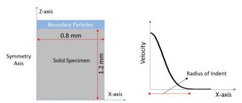
Figure 3. The figure on the left show the computational domain for solid simulation, the boundary particles marked in blue are given a downward velocity plotted on the right. (a Gaussian distribution is provided as the indent velocity as shown on the right, the radius of indent is defined as the distance from the center where the velocity is 1% of the peak value, a constant velocity is given to the indenter wrt time)
