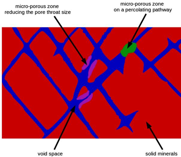
**Fig. 1** Schematic of a micro-CT rock sample image. The *red* and *blue* regions are identified as solid minerals and void spaces, respectively. The *green* and *purple* areas denote microporous regions
