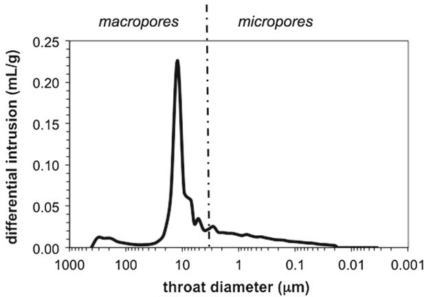
**Fig. 2** Pore-throat size distribution of the studied Berea sandstone determined from a mercury-injection test (presented as the differential intrusion). The limit pore-size separating macropores and micropores in this study (3.16 microns) is displayed as a *dashed line*
