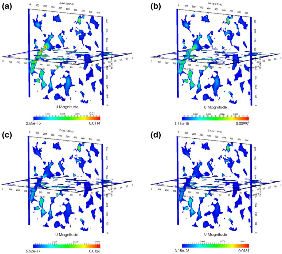
**Fig. 7** Plot of the velocity distribution for different sub-voxel porosity values: **a**  $\epsilon_{\text{micro}} = 1$ , **b**  $\epsilon_{\text{micro}} = 0.9$ , **c**  $\epsilon_{\text{micro}} = 0.5$ , **d**  $\epsilon_{\text{micro}} \approx 0$
