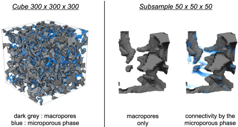
**Fig. 4** Three-dimensional representation of the connected macroporosity and microporous phases on a cube of  $300 \times 300 \times 300$  voxels (*left*) and close-up of macropores that are only connected through microporous material (*right*)
