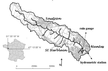
Figure 1. Chezine catchment indicating the location of the rain gauge and the hydrometric station at the outlet. The grey areas correspond to the urban database layers superposed (roads and buildings).
