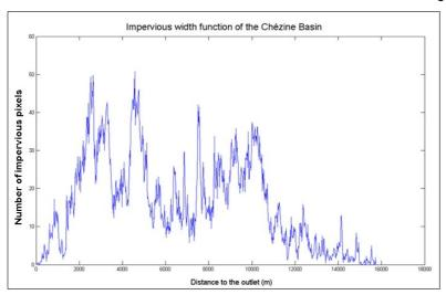
Figure 8. The Impervious width function of the Chézine basin
