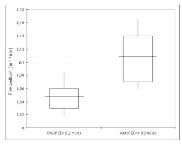
Figure 6.: Flow coefficient values for dry events (PED <0.2 m3/s) and for wet events (PED>=0.2 m3/s). The bars represent the interval of values for 50% of the events. The vertical extension lines represent the edges for 80% of the events. The horizontal lines represent the mean FC value of each group.
