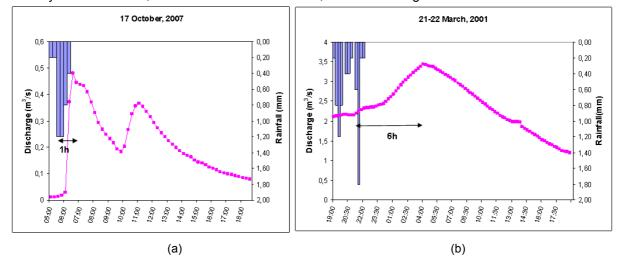
Figure 2. Observed discharge (m3/s) in pink lines and averaged 15 min observed rainfall (mm) represented by blue bars on (a) 17 October 2007 and (b) on the 21st -22nd of March 2001. The time-lag is indicated by double arrows.
