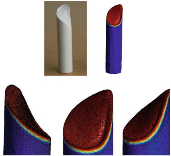
Fig. 17 Chalk comparison of the final state between simulation and experiment presented in Bordas et al. (2008) (Reprinted from Bordas et al. (2008) Copyright (2007) with permission from Elsevier)
