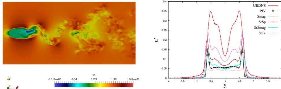
**Figure 1** Cylinder wake flow LES simulations based on location uncertainty principle: (Left), Velocity norm for the LES with the StSP subgrid tensor; (Right), Streamwise velocity fluctuation profiles at 1.06D behind the cylinder axis, for different subgrid tensor models compared with PIV of [3] and an under resolved DNS.
