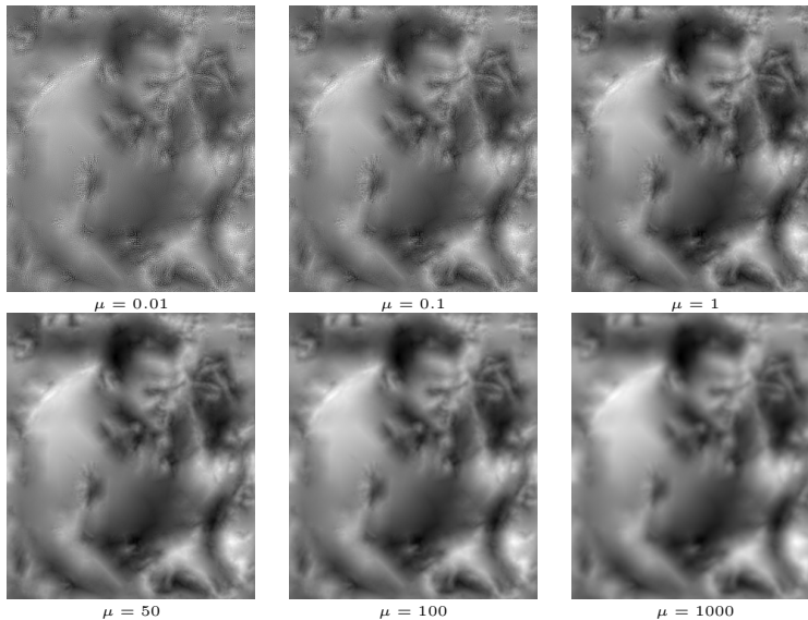
Figure 5: Influence of the regularization parameter \mu in MS-Poisson. As expected, increasing \mu penalizes more the L^2 -norm of the gradient and thus makes the image blurrier. We empirically observed that a good compromise between recovered details and smoothness is often attained around \mu = 50 . (Images are better seen on the electronic version)
