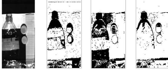
Fig. 1: Example of the fusion impact on classification rate (Superposition board). From left to right: test board image, binary representations of the well classified pixels (in white) considering  $S_1$ ,  $S_2$  and their evidential fusion, respectively.
