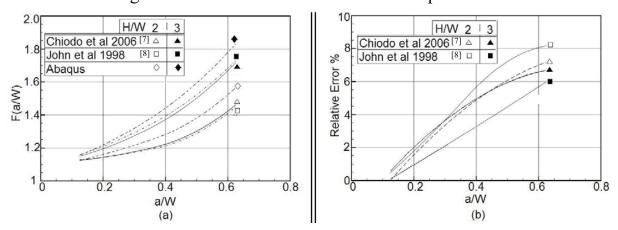
Figure 4. (a) Variation of correction factor F(a/W) vs. a/W at two H/W ratios. (b) Relative error of F(a/W) estimation between ABAQUS® and [7] and [8]
