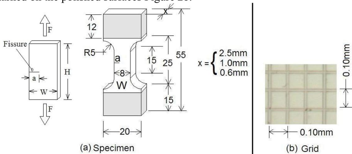
Figure 2. Specimen geometry and engraved grid on specimen surface.
