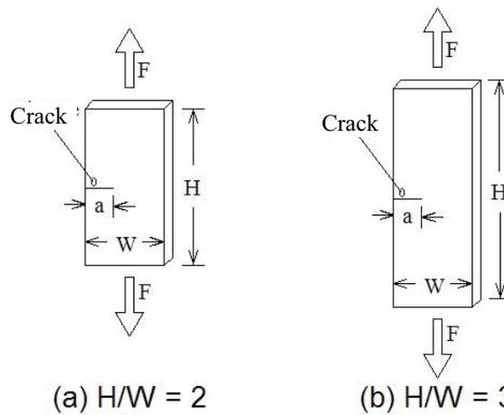
Figure 3. Schematic of the SET standard specimens.
