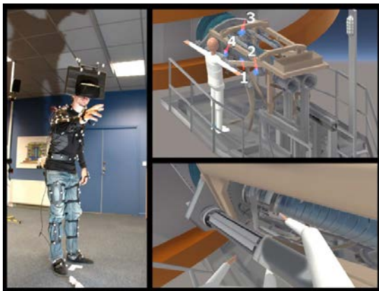
Figure 1: Left. A subject in the experimental setup. Top right. Global view of the experimental VE: avatar in the initial position and targets. Bottom right. First person view inside the HMD.
